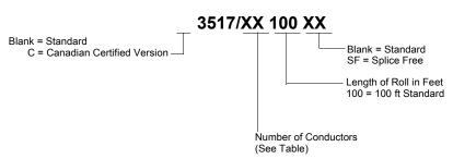
Note: Contact 3M for availability of additional conductor counts and/or custom roll lengths.
